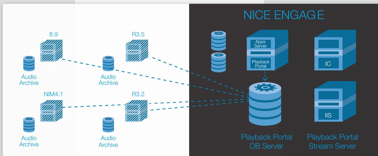
The key is the ability to playback legacy recordings directly from within the NICE Engage platform. One server, the Stream Server (with IIS Media Services), handles all playback requests and hosts the Playback Portal services, while the other, the Database Server, is dedicated to legacy databases.
